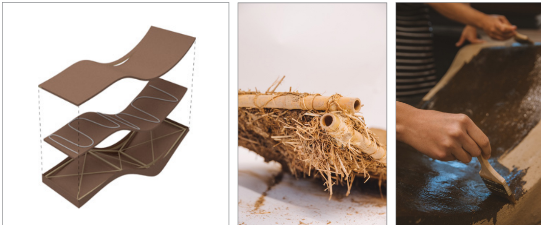
Figure 3. The process of designing and constructing Jandug, using a layered skeleton building, a light straw clay infill, and a cob finish sealed with flaxseed oil. Research Students: Bisher Tabbaa and Sarah Hejazin.
