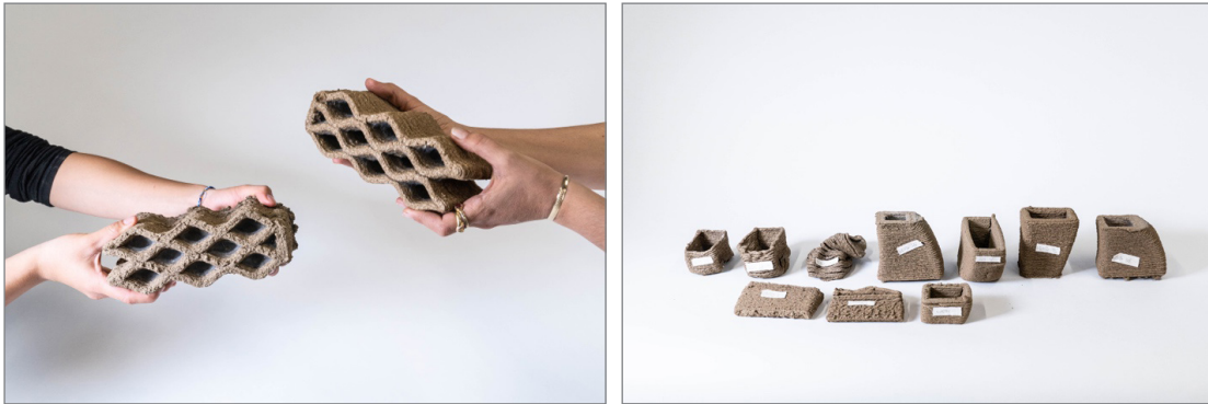
Figure 2. 3D printed prototypes of cob, light cob, and light straw clay. Research Student: Zackary Bryson.
