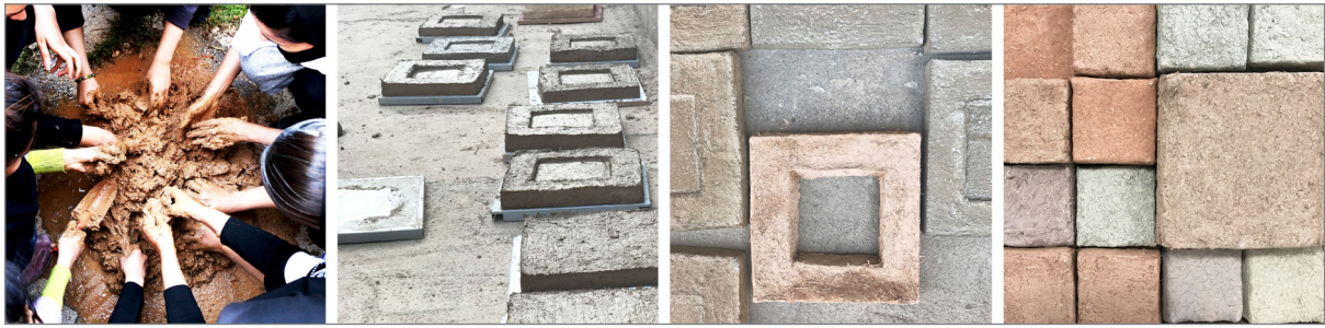
Figure 1. The first step of making these adobe is blending clay and straw then adding water. The mixture is kneaded well, finally it is molded in frames and dried in shadow. Some adobes in small size have been made for plaster color tests.
