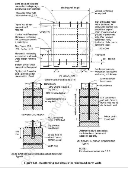
REINFORCED EARTH WALLS PER THE NEW ZEALAND CODE Excerpt from NZS 4299.
