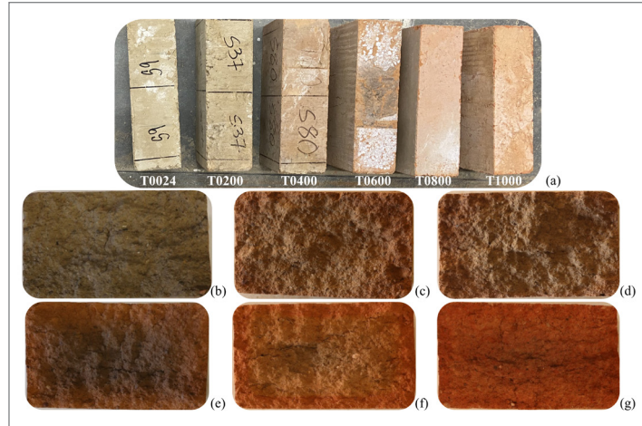
Figure 3. Visual inspection: (a) CSEB specimens after exposure to different temperatures, (b-g) typical cross-sections of CSEBs after exposure to 24 °C, 200 °C, 400 °C, 600 °C, 800 °C, and 1000 °C.
