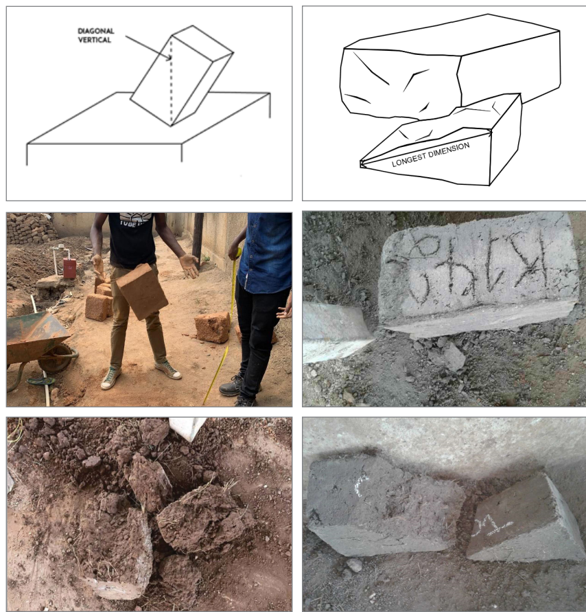
Figure 2. (top left) diagram showing drop test, (top right) dimension measured after drop test, (middle left) drop test in action, (middle right) block that passed drop test, (bottom left) block that failed drop test because it shattered, (bottom right) block that failed drop test because the measured dimension was too great.
