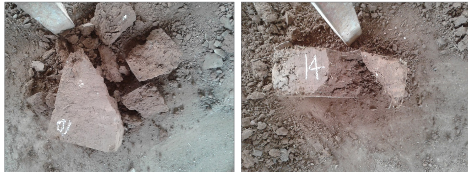
Figure 6. Representational images of Phase 2 drop test results with blocks made with Gasabo soil. Right: control blocks without fibres. Left: blocks with 5kg/m 3 of 5-7cm long Ishinge fibres.
