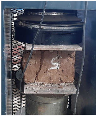
Figure 1. Compressive strength testing of adobe blocks.
