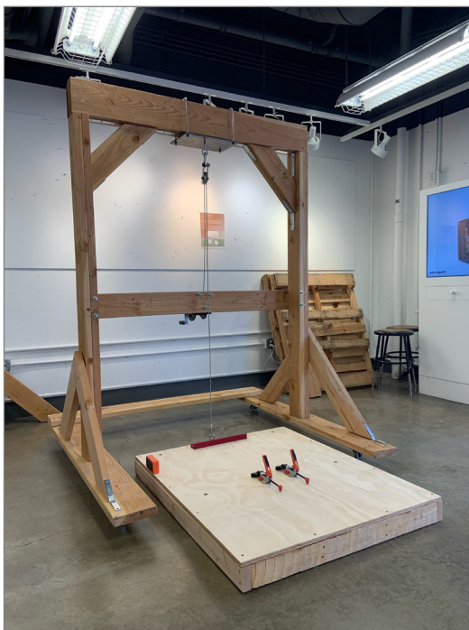
Figure 5. Manually operated lateral tilting table test machine.
