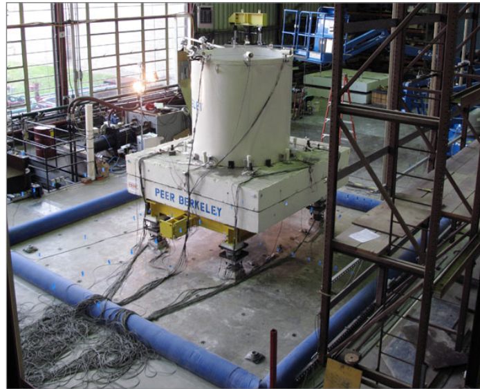
Figure 2. UC Berkeley PEER Earthquake Shaking Table. Photo: UC Berkeley Pacific Earthquake Engineering Research Center
